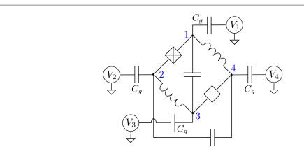
**Figure 6.**  $0-\pi$  circuit coupled capacitively to voltage sources  $V_i(t)$ , as used in the modeling of charge noise.
