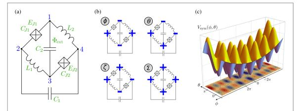
**Figure 2.** (a)  $0-\pi$  circuit diagram, consisting of two Josephson junctions, two large inductors and two large capacitors. (b) Schematic representation of the normal modes of the linearized circuit (no parameter disorder), which define the new circuit variables  $\phi$ ,  $\theta$ ,  $\zeta$  and  $\Sigma$ . (c) Potential energy of the disorderless  $0-\pi$  qubit.
