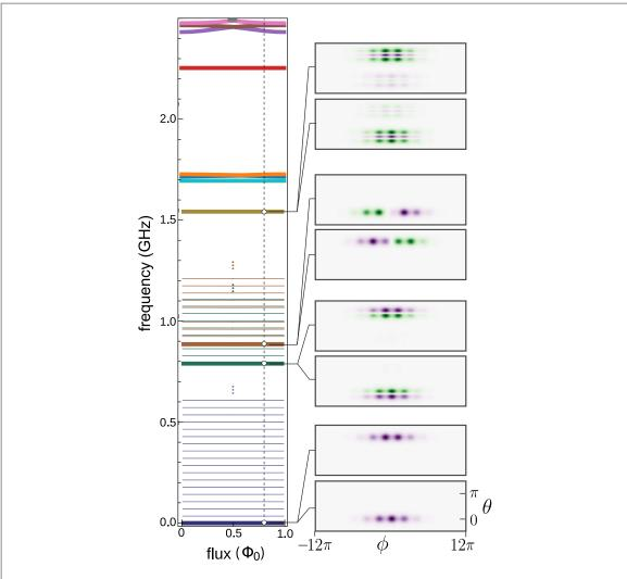
Figure 3. Energy spectrum of parameter set 1 (see table 1), plotted as a function of flux, along with a few selected  $0-\pi$  wave functions calculated at  $\Phi_{\rm ext}=0.8~\Phi_0$ . (Only a limited number of  $\zeta$ -mode excitations is shown.)
