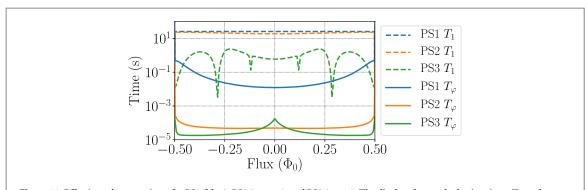
**Figure 11.** Effective coherence times for PS1 (blue), PS2 (orange), and PS3 (green). The displayed pure-dephasing times  $T_{\varphi}$ , and depolarization times  $T_1$  are obtained from the cumulative rates combining all processes described in section 4.
