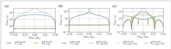
Figure C1. Purcell depolarization times obtained for parameters (a) PS1, (b) PS2 and (c) PS3. Results obtained by numerically are shown in solid, colored lines, while using perturbation theory in black, dashed, dotted and dashed-dotted lines.
