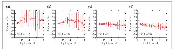
Figure 3. Performance of rate extraction algorithm. We show the percentage deviation of the extracted mean transition rate  $(\Gamma_{\uparrow} + \Gamma_{\downarrow})/2$  from the true mean transition rate as a function of the extracted mean rate, as determined from roughly 7000 simulated data sets. Error bars show the root mean squared error. The four panels correspond to four different values of the initial SNR, as described in the text.
