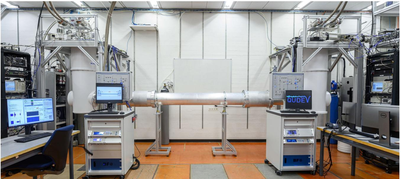
FIG. S6. Photograph of the experimental setup during operation. The dilution refrigerator units, whose vacuum cans appear as white vertical cylinders, are connected to each other by the cryogenic link (long horizontal aluminum cylinder). The superconducting qubits and the cold waveguide are housed inside the dilution refrigerator units and the cryogenic link, respectively. The electronic instruments are stored in two black racks seen on the far sides of the picture.
